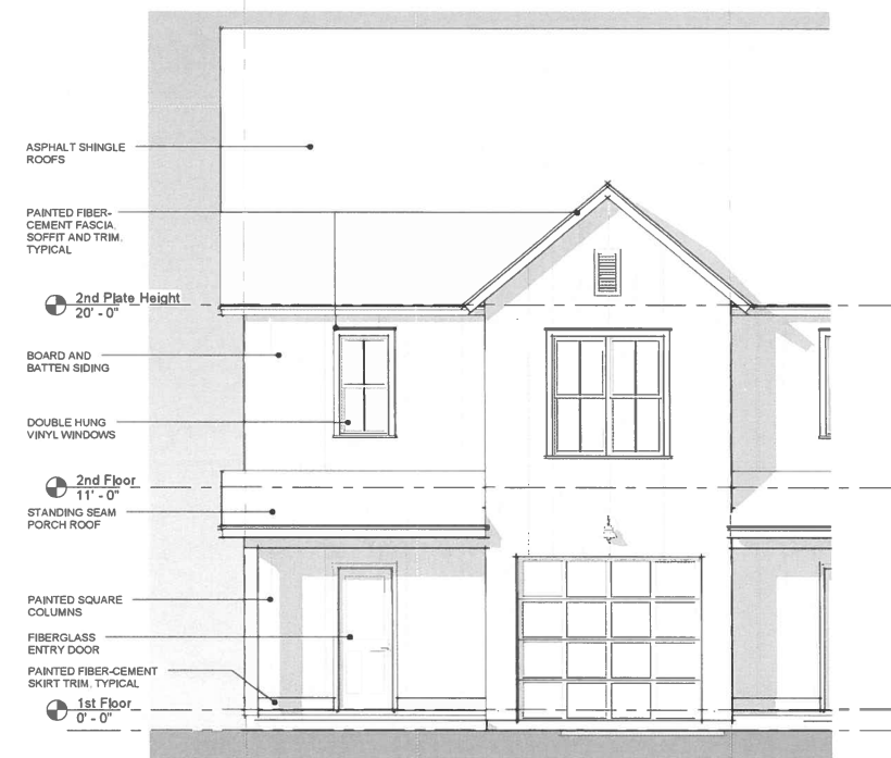
4 | Townhouse Unit - Enlarged Front Elevation 1/4" = 1'-0"
