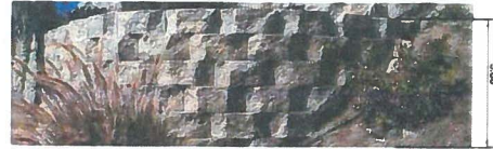
PROPOSED SPLIT FACED CONCRETE MODULAR RETAINING WALL WITH VARYING HEIGHT (MAX 5') SCALE: N.T.S.
